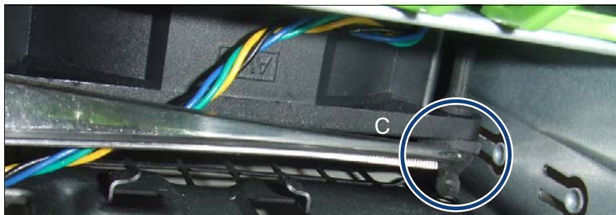
Figure 90: Fitting front fan rivet C
